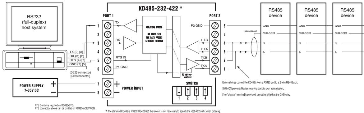
Another application is a multi-drop connection of non-addressable RS232/422/20mA devices, to enable them to be conveniently polled from a single RS485 Master device. The KD485-ADE can act as an "addressable adapter".
